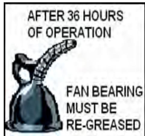
**fully re-greased at site by maintenance contractor** after installation and commissioning.
